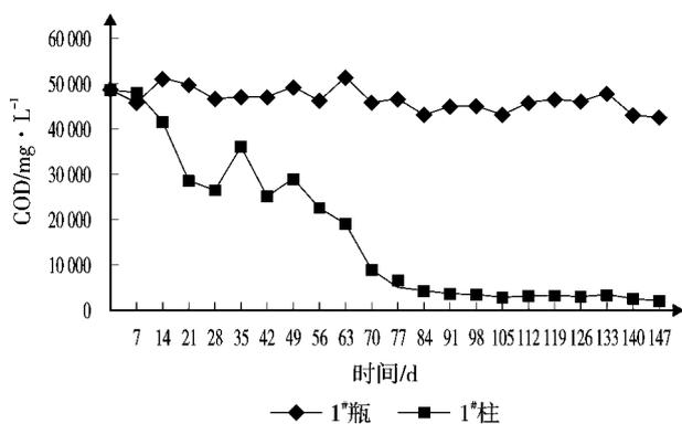
图 4 1<sup>#</sup>瓶和 1<sup>#</sup>柱渗滤液的降解曲线
